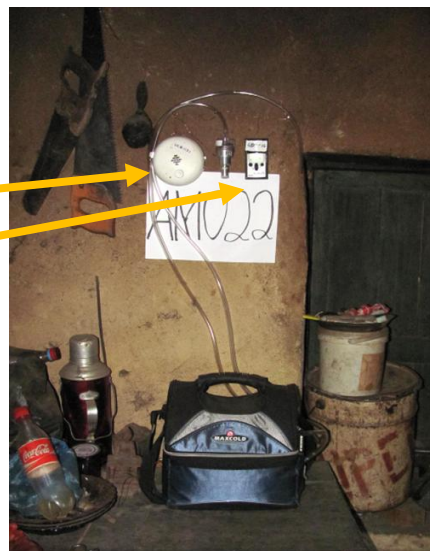
Figure 8: HAP monitoring equipment in kitchen PM Monitor CO Monitor
