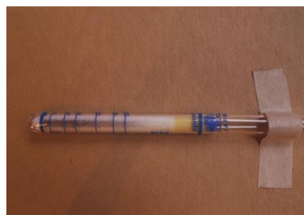
Figure 9: Individual CO tube
